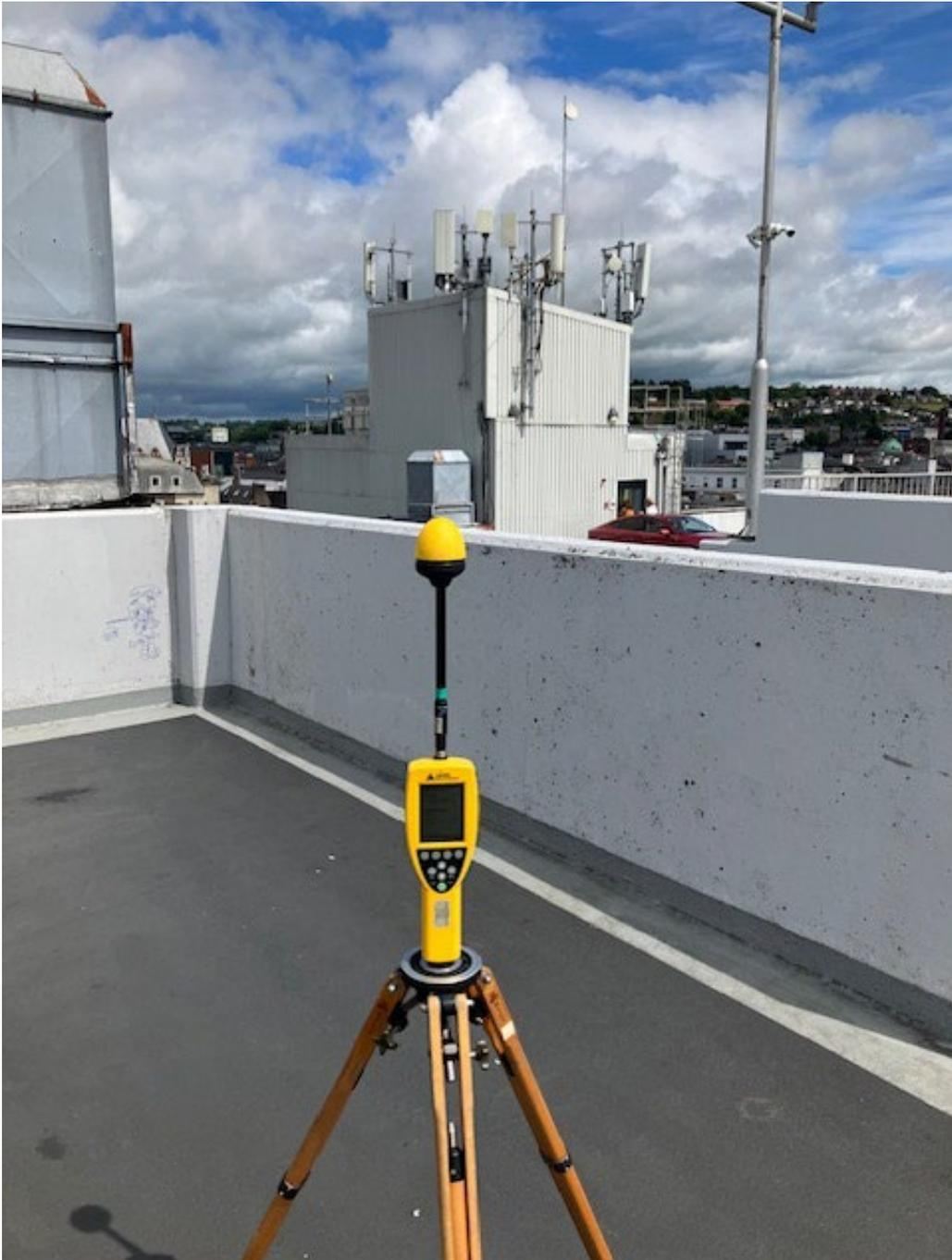
**Photo 1. Broadband Measurement location looking towards antennas**
