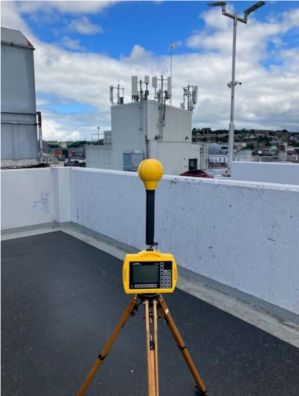
**Photo 2. Frequency selective measurement location looking towards antenna**
