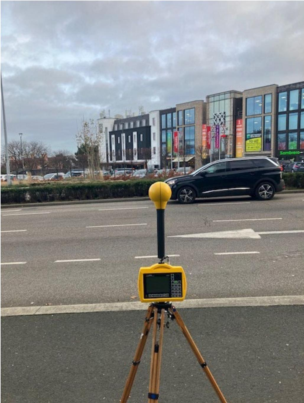
**Photo 2. Frequency selective measurement location looking towards antennas**
